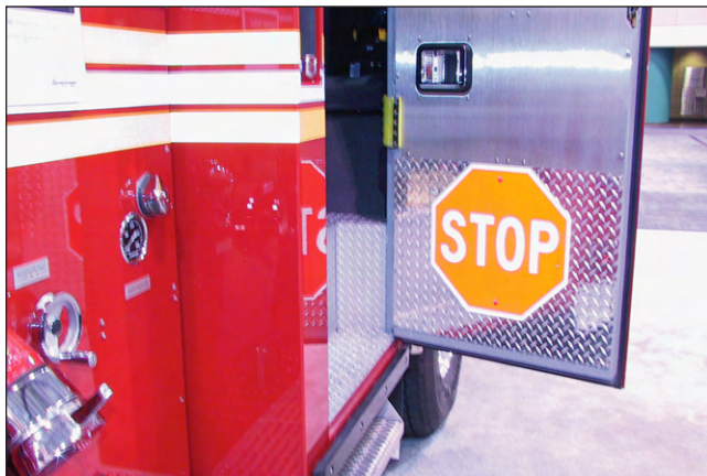
Figure 3.22—Some department use reflective stops signs on the insides of doors as opposed to striping.
