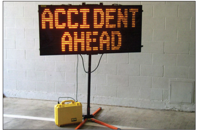
Figure 3.4a—Fire departments may carry portable electronic message boards. Courtesy of Ron Moore, McKinney, TX FD.
