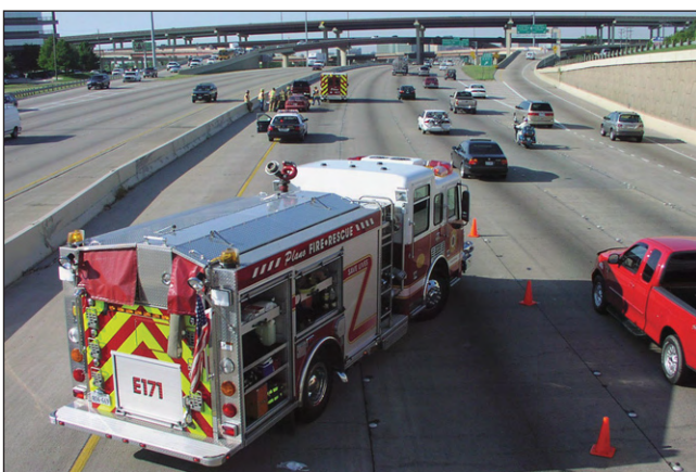
Figure 6.3—The first apparatus on the scene should assume a blocking position. Courtesy of Ron Moore, McKinney, TX FD.
