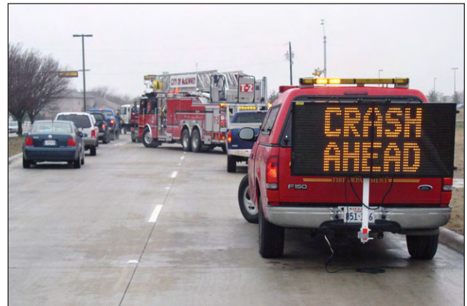
Figure 3.4b—This portable electronic message board is mounted to a vehicle trailer hitch. Courtesy of Ron Moore, McKinney, TX FD.
