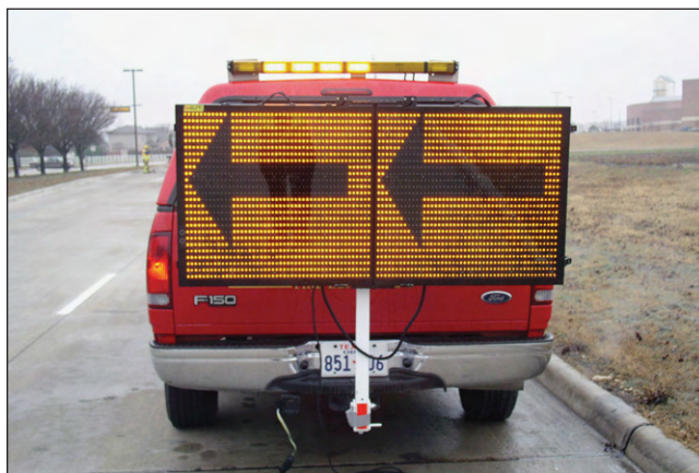
Figure 3.13a—The command vehicle has a trailer hitch-mounted LED arrow board. Courtesy of Ron Moore, McKinney, TX FD.
