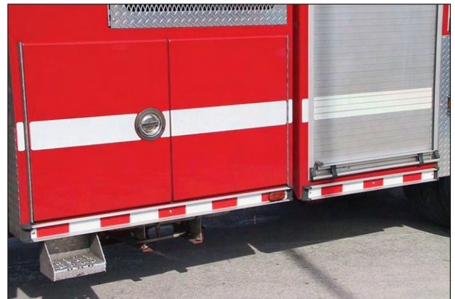
Figure 3.23—The use of DOT-style reflective trim in apparatus rub rails is an expensive way to increase apparatus visibility.
