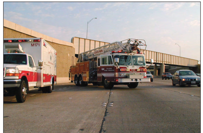
Figure 4.2—Park the apparatus in a manner that shields the work area.
