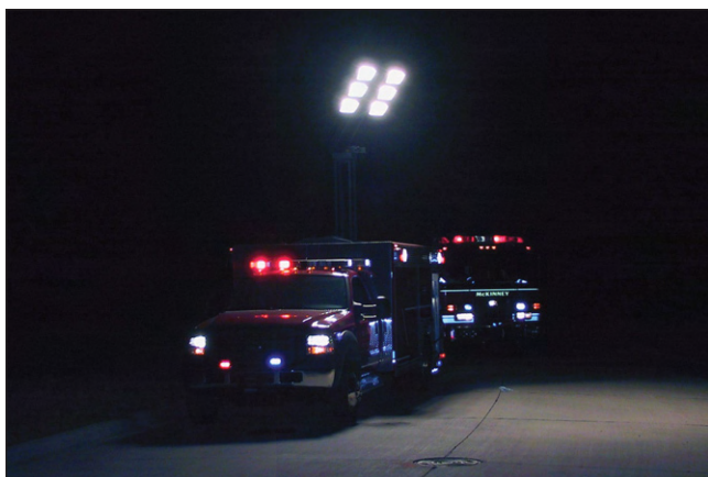
Figure 4.7—Make sure lights are deployed in a manner that is not blinding to approaching motorists.
