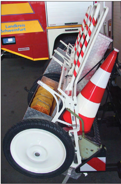
Figure 3.27 –Traffic control carts are clipped to the back of German fire apparatus and can be deployed by a single firefighter.
