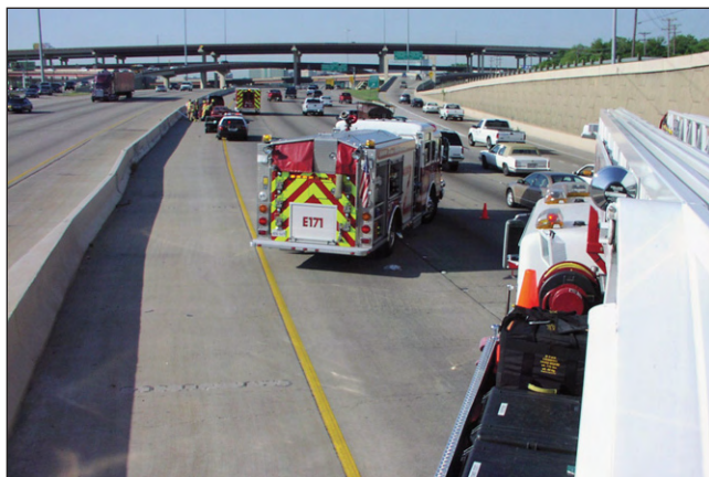
Figure 4.5—Place apparatus between the flow of traffic and the work area. Courtesy of Ron Moore, McKinney, TX FD.
