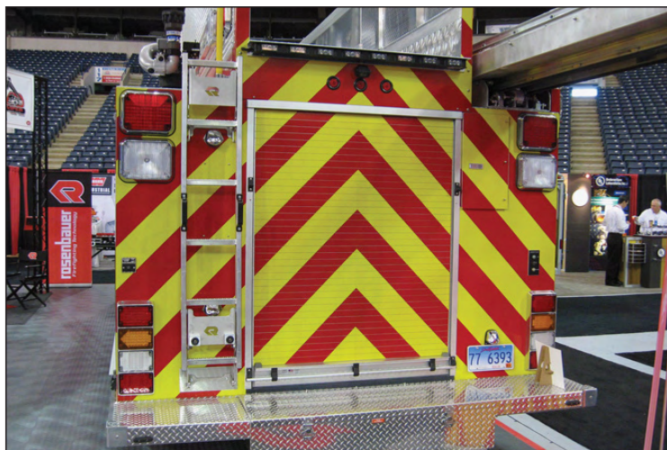
Figure 3.25—Many U.S. apparatus now sport reflective markings on the rear of the vehicles.
