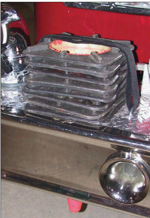
Figure 3.8—This department designed a place to store traffic cones in the extended front bumper of the apparatus.
