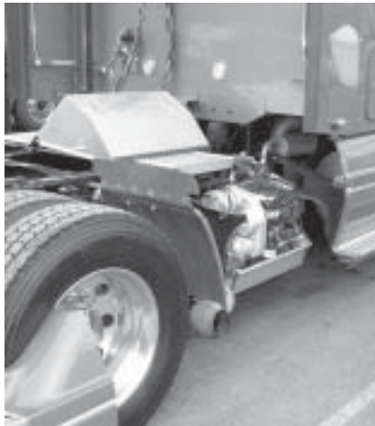
A small diesel engine like that pictured here should pay for itself in fuel savings if it replaces the need to idle the full-size truck engine. Photo courtesy of Willis APU/Auxiliary Power Dynamics
