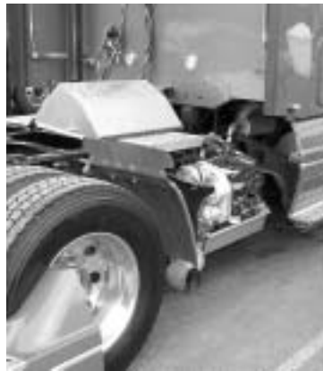
A small diesel engine like that pictured here can pay for itself in fuel savings as it replaces the need to idle the full-size truck engine. Photo courtesy of Willis APU/Auxiliary Power Dynamics
