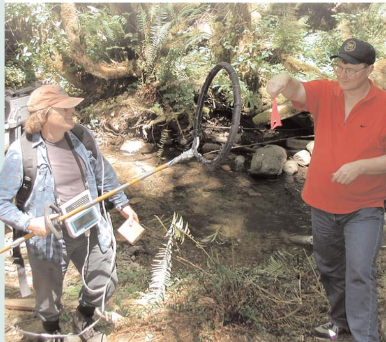
Doug Bateman and Arne Skaugset illustrate PIT tag technology using a mobile antenna.
