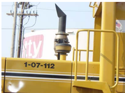
DOC on construction equipment
