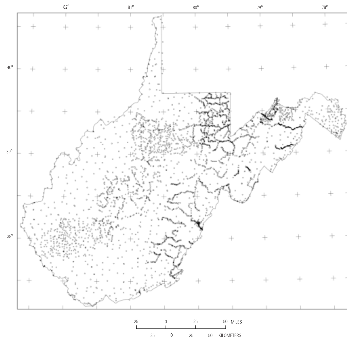
Figure 4. Distribution of the 4,092 gravity measurement stations used to compile the Bouguer gravity map, figure 3.
