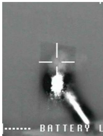
Figure4-13d. Standard and Infrared Video Images of Gerb Discharge onto a Non-fire Retarded Polyurethane Foam Sheet on Gypsum Board Wall at t = 2 seconds.
