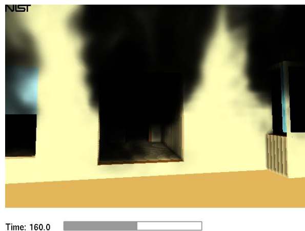
Figure 5-49. Heavy smoke leaving front door and open main bar window (160 seconds)
