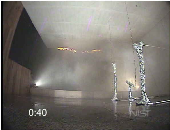
Figure 5-24. Suppression with three sprinklers operating in each case, t = 40 seconds after ignition.
