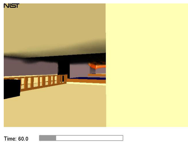
Figure 5-46. Smoke beginning to roll across ceiling (video 53 seconds, simulation 60 seconds)
