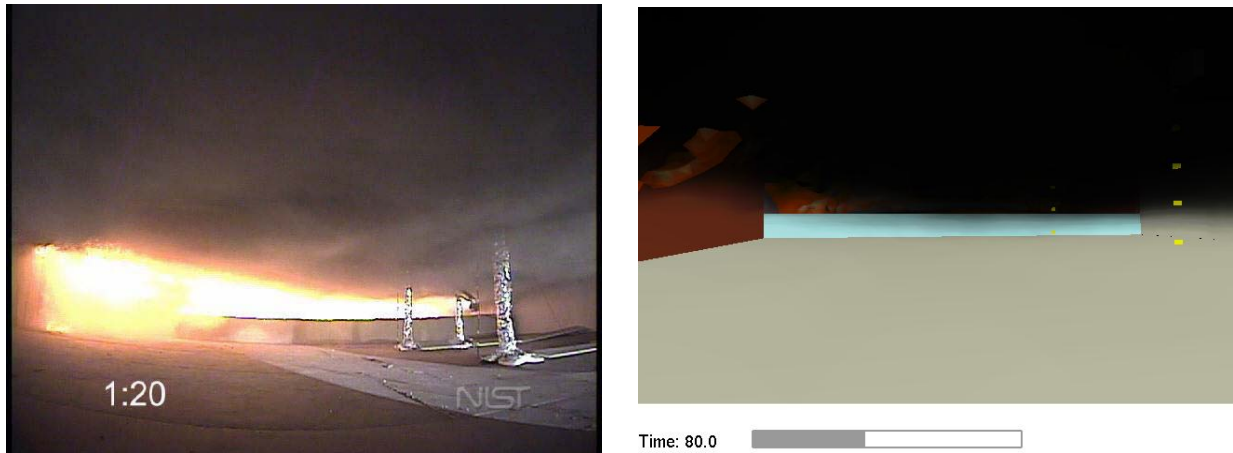
Figure 5-10. Fire continues to spread, t = 80 seconds after ignition.
