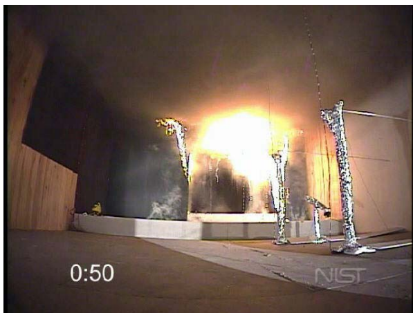
Figure 5-7. Ceiling of alcove fully involved in fire, t = 50 seconds after ignition.
