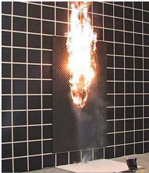
Figure 4-13h. Standard and Infrared Video Images of Gerb Discharge onto a Non-fire Retarded Polyurethane Foam Sheet on Gypsum Board Wall at t = 30 seconds.
