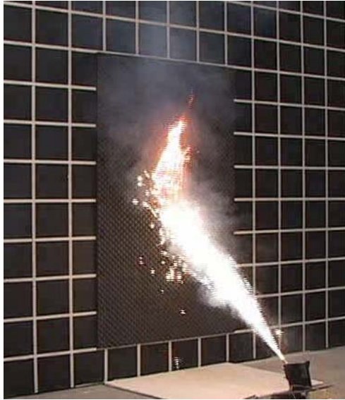
Pyrotechnic device impinging on non-fire retarded polyurethane foam panel
