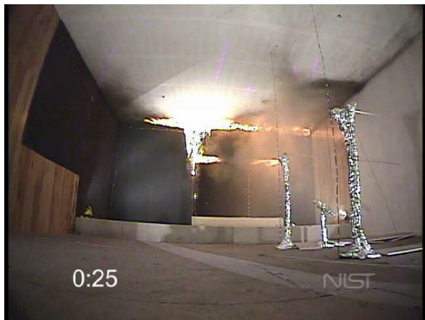
Figure 5-22. Initial sprinkler operating, t = 25 seconds after ignition.
