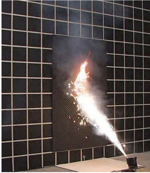
Figure 4-13g. Standard and Infrared Video Images of Gerb Discharge onto a Non-fire Retarded Polyurethane Foam Sheet on Gypsum Board Wall at t = 15 seconds.
