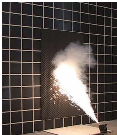
Figure4-13d. Standard and Infrared Video Images of Gerb Discharge onto a Non-fire Retarded Polyurethane Foam Sheet on Gypsum Board Wall at t = 2 seconds.
