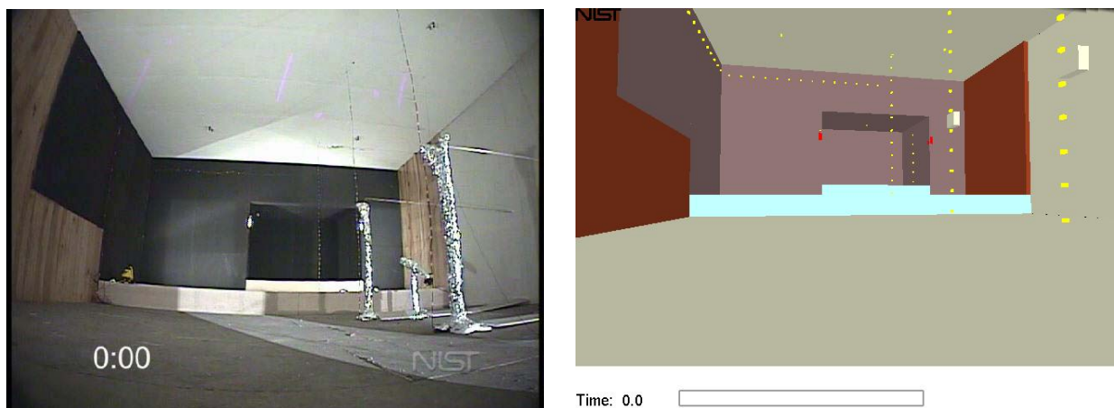
Figure 5-2. Ignition at the corners of the drummer's alcove, t = 0 second.
