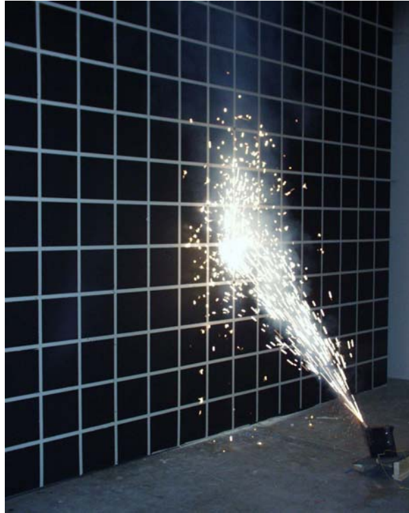
Figure 4-11. Single Gerb at 45 degrees and in a Plane Perpendicular to Wall.
