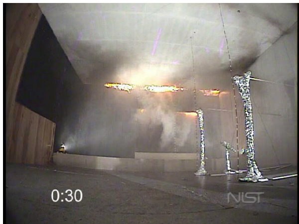
Figure 5-23. Third sprinkler operating in experiment, t = 30 seconds after ignition.
