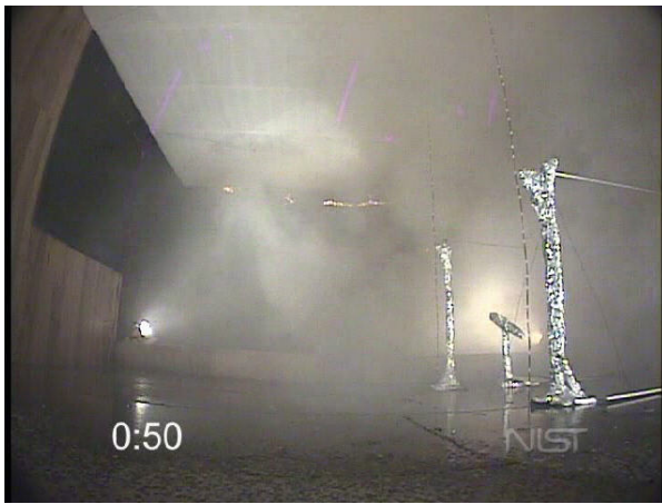
Figure 5-25. Fire suppression continues in both the experiment and the simulation, t = 50 seconds after ignition.
