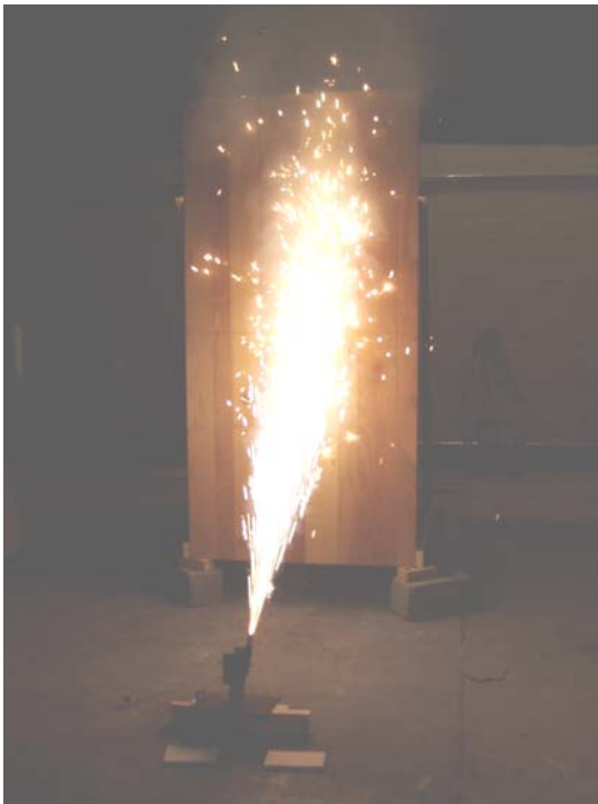
Figure 4-14a. Gerb impinging on wood panel.
