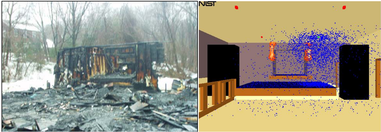
Remains of the platform area after the fire (left) and an image from the simulation of The Station fire had sprinklers been installed (right)
