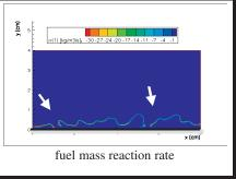
Direct numerical study of flame-wall interactions and wall heat transfer. Instantaneous snapshots allow a detailed observation of flame-extinction events.
