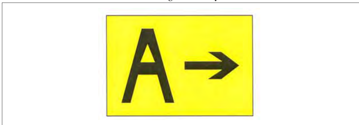
FIG AD 1.1-45 Direction Sign for Runway Exit
