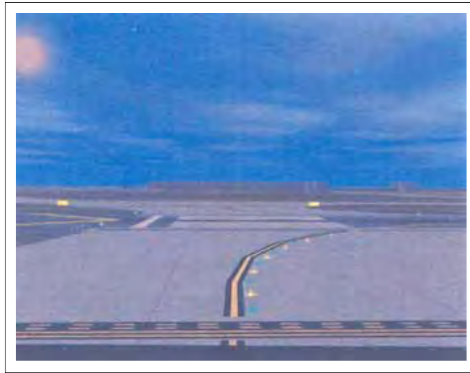
FIG AD 1.1-9 Taxiway Lead-On Light Configuration
