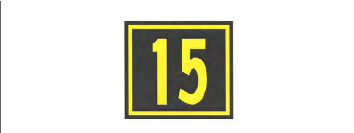
FIG AD 1.1-41 Runway Location Sign
