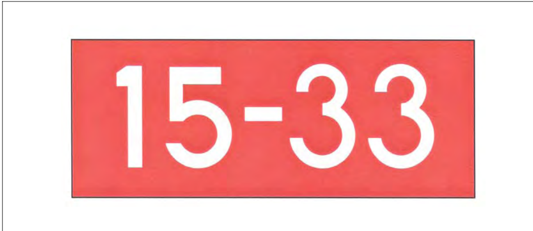
FIG 2-3-24 Runway Holding Position Sign
