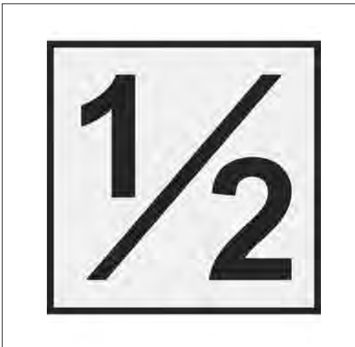
FIG 7-5-1 Typical Runway Half-way Sign
