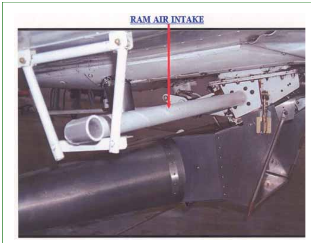
FIGURE 3-10-13 Dry Material Application System - RAM Air Intake
