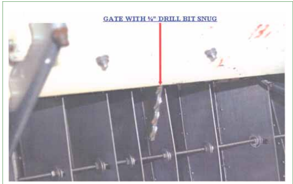
FIGURE 3-10-18 Proper Gate Opening Size With Drill Bit
