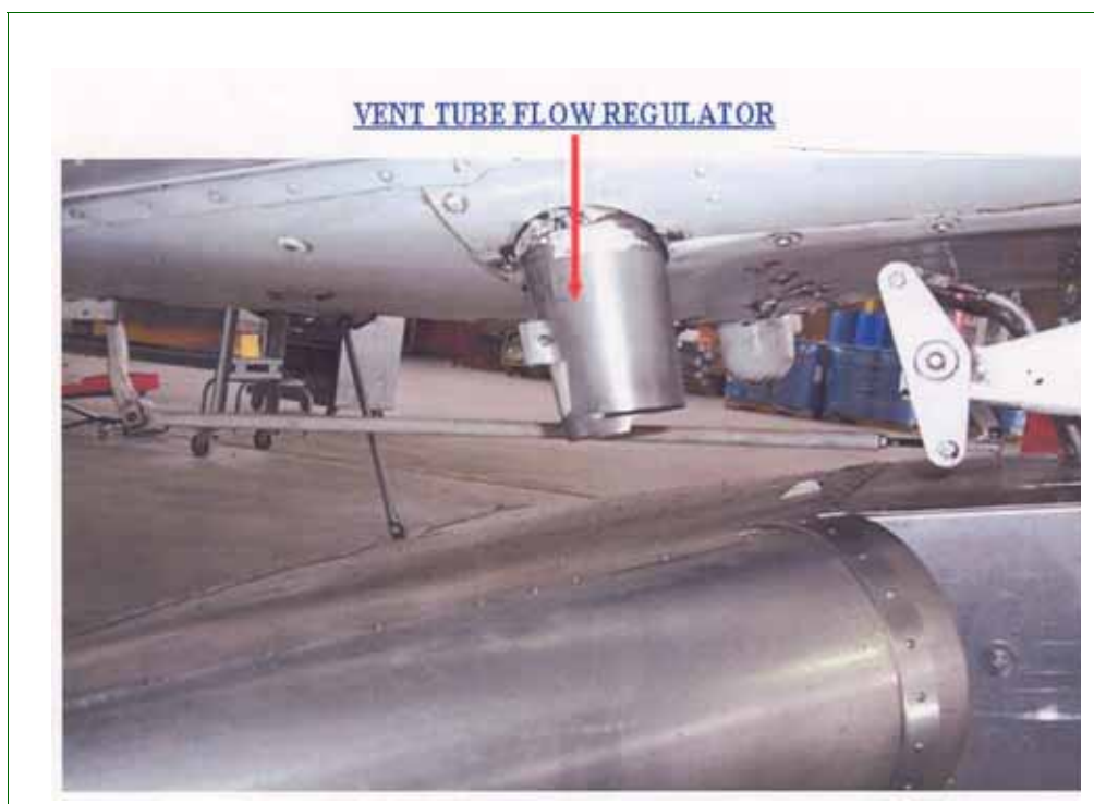
FIGURE 3-10-15 Dry Material Application System - Vent Tube Flow Regulator
