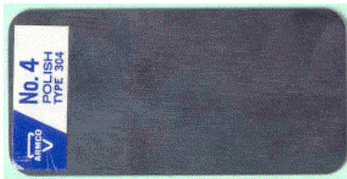
Photo 2 - Stainless Steel Type 304, No.4 Polish is exceptionally uniform normally used without further finishing. This is the established standard for dairy and food processing equipment because it is easy to keep clean and sanitary.
