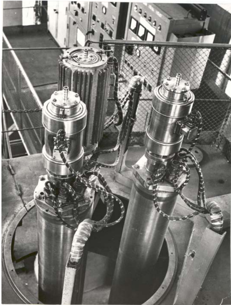
FIG. 5. Sodium rig for testing of drives, control and safety system rods for the BN-600.
