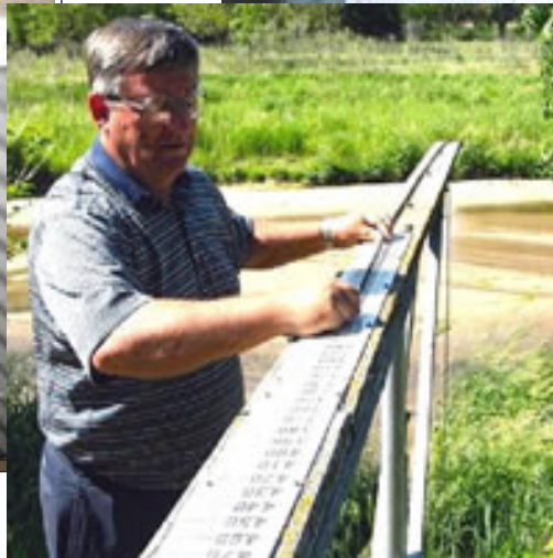
Delmar stretches the chain to get a reading on the chain gage.
