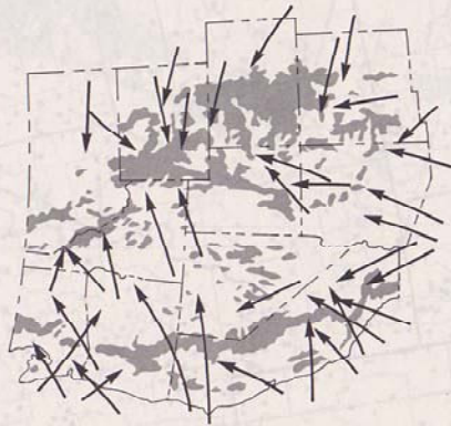
Figure 7. Principal path of moisture inflow in the western United States for storms producing large precipitation amounts. Toned areas are major orographic barriers.
