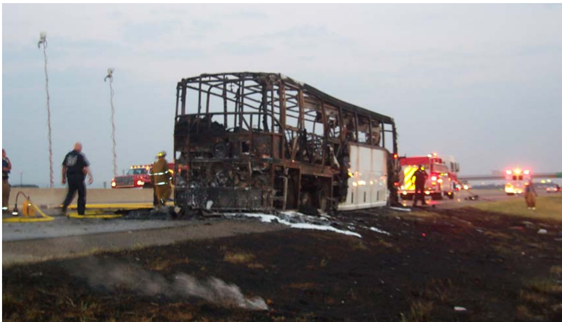
Figure 3. Damaged motorcoach on I-45 following fire.
