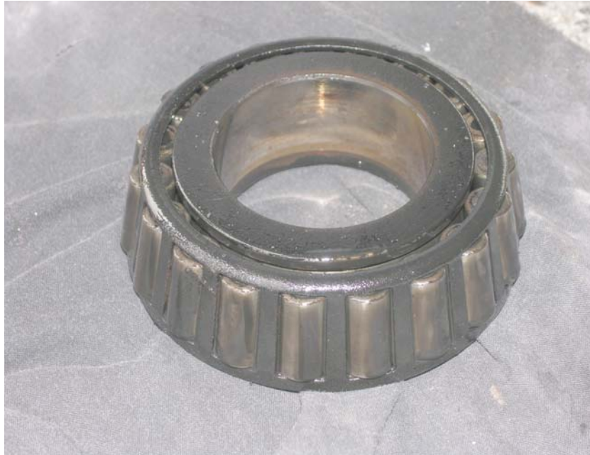
Figure 13. Left tag axle outer wheel bearing assembly.
