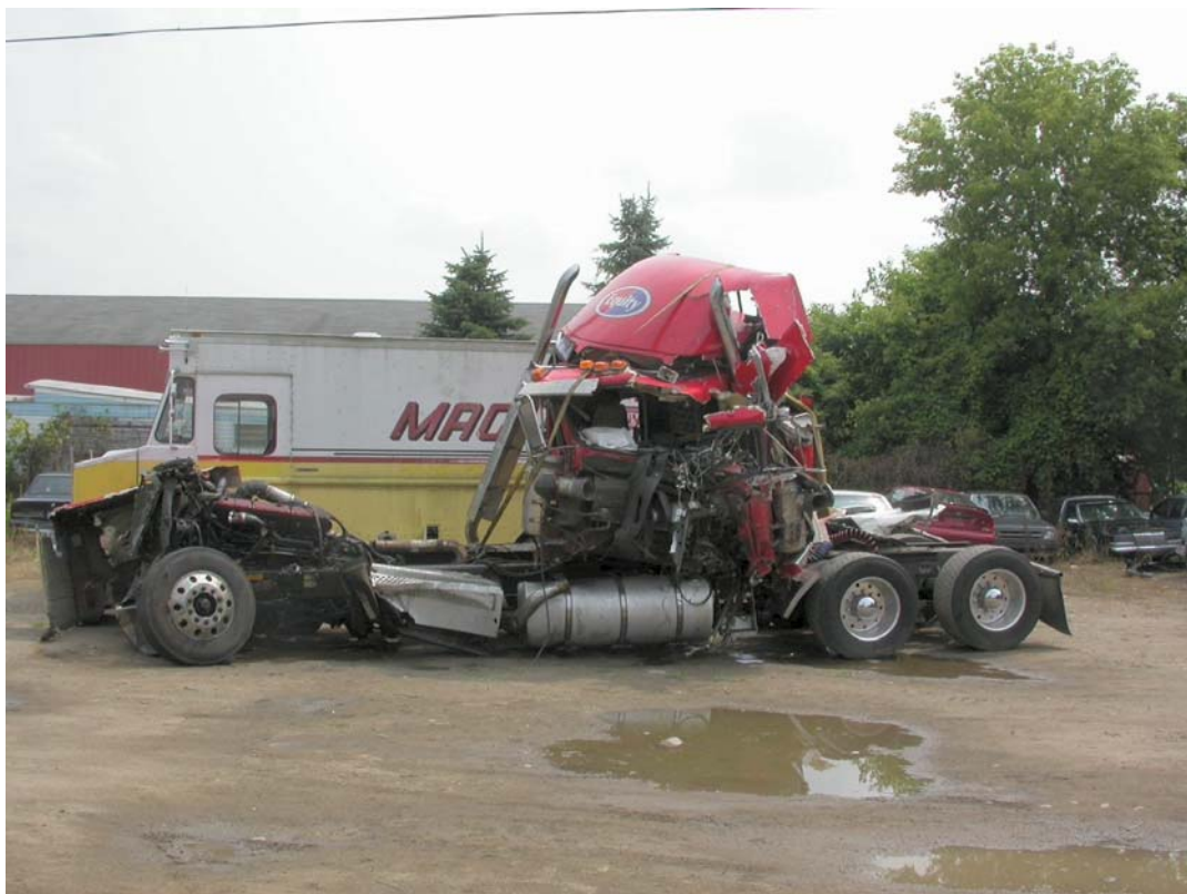
Figure 2. This postaccident lateral view of the Kenworth tractor shows the extent to which the cab was crushed rearward. The front of the tractor is on the left.
