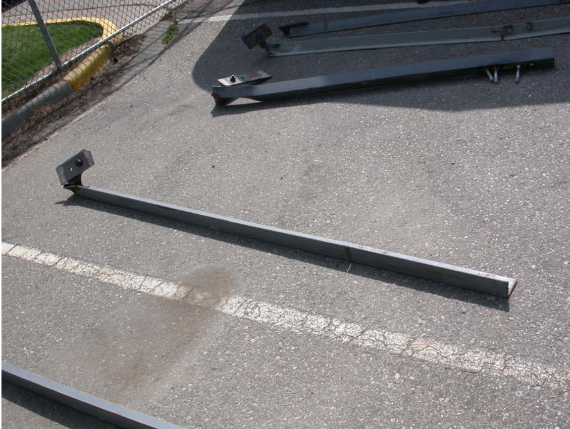
Figure 3. Postaccident photograph of one of the angle-shaped steel braces used to brace the accident girder.
