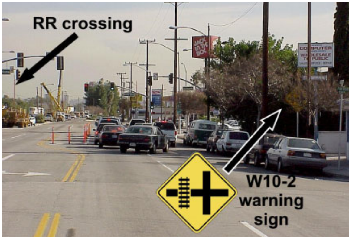
Figure 5. Obscured advance warning sign.
