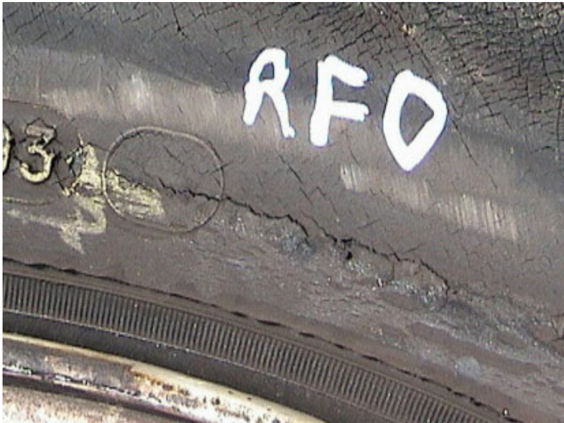
Figure 16. Right front tire sidewall cracking.
