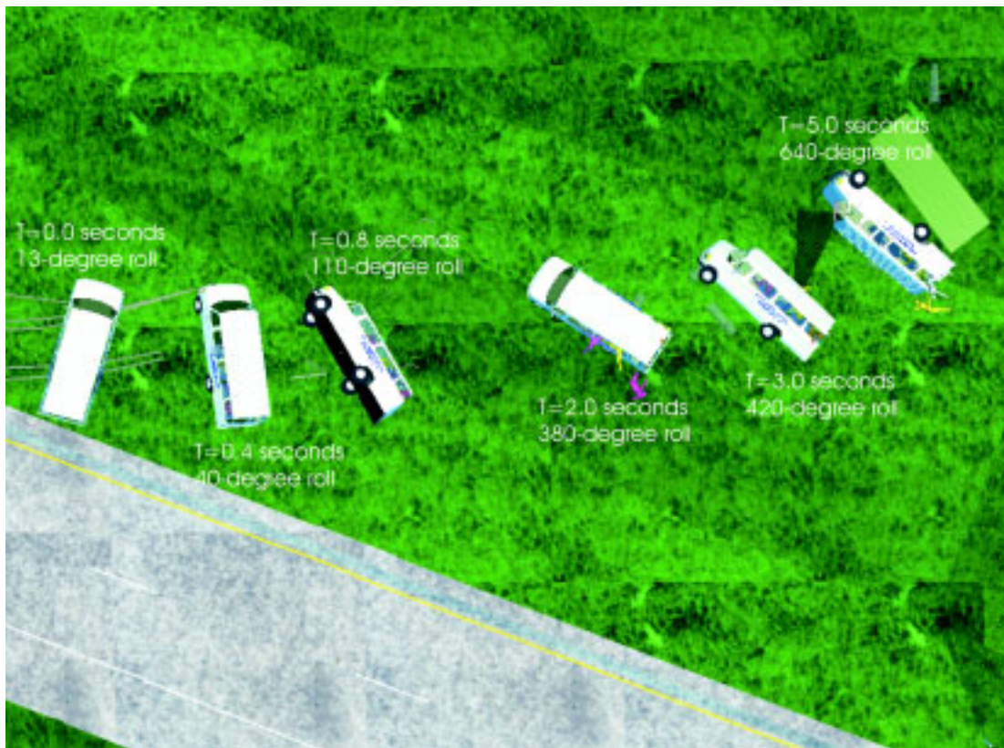
Figure 20. Potential path of the van during the overturn; the time is based on the beginning of the rollover.
