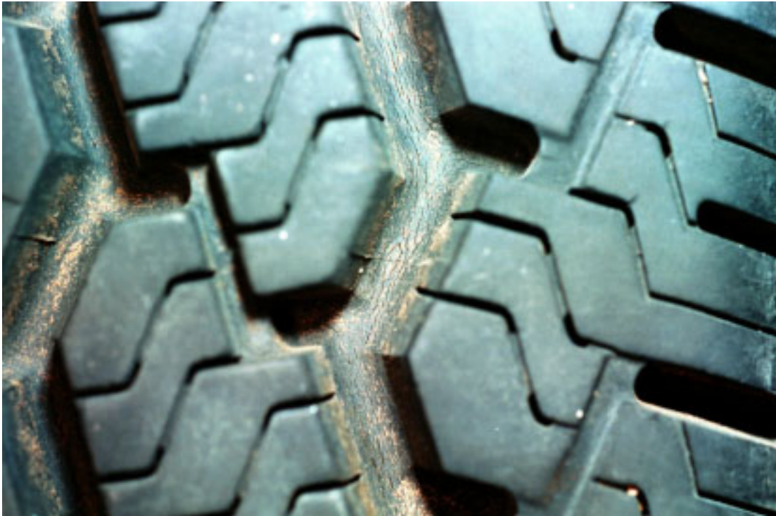
Figure 5. Left front tire tread groove cracking.
