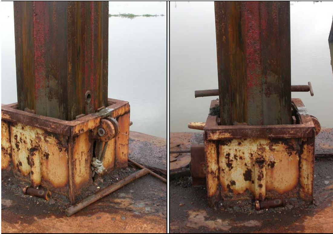
Figure 11. Photos showing spud with securing pin lying alongside (left) and with securing pin inserted (right).
