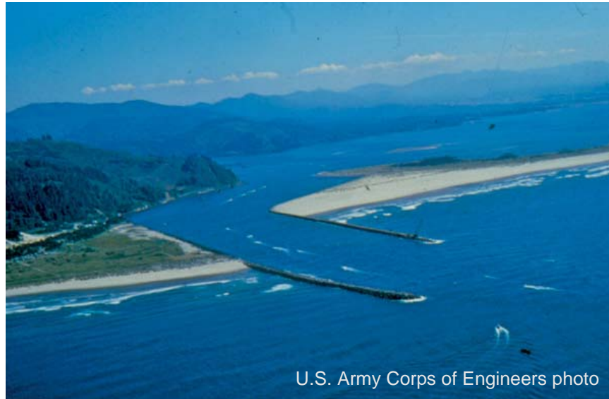
Figure 2. Looking southeast from Pacific Ocean toward Tillamook Bay, with inlet between north jetty (left) and south jetty (right). The Tillamook bar, not shown, is west of the jetty tips. The Taki-Too capsized outside the tip of the north jetty and washed up on the sandy beach on the left of the photo.
