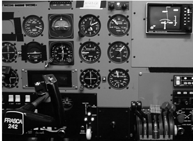
Figure 1: Frasca 242 Simulator Instrument Panel Avidyne 5RR display is located at the upper-right corner (Map VNAV format is in use).
