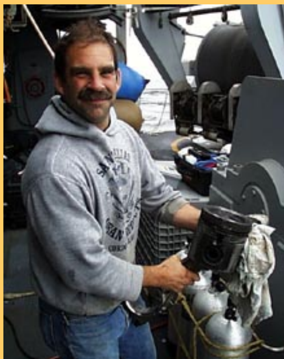
Chief Mate Dave Bayard shows the blown piston from Discovery Bay's main diesel engine.
