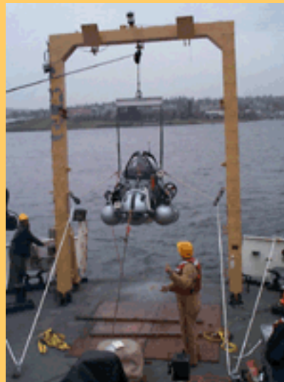
DeepWorker launched by crane on the McArthur
