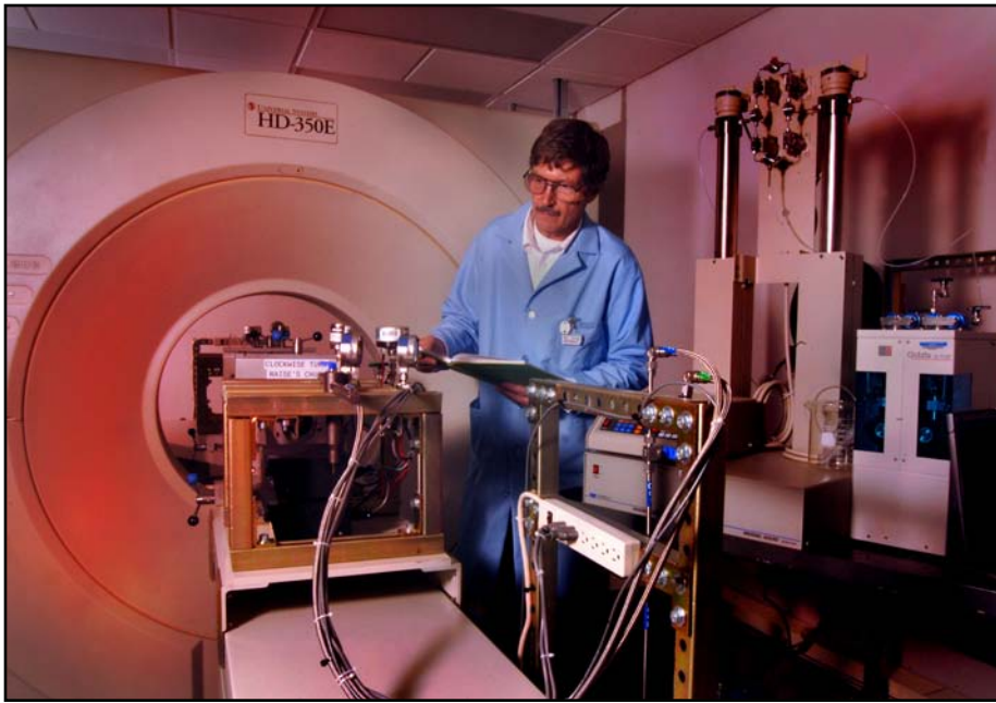
Robert McLendon adjusts the CT scanner used during research at NETL. The scanner is used mainly to measure in-situ fluid displacement and sorption of fluids within mineral cores
