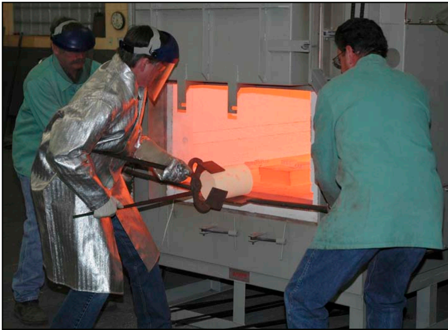
The prototype ingot made from Armstrong Process titanium is being removed from the preheat furnace for hot working.
