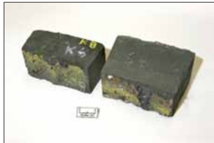
NETL-developed refractory (right) showing improved performance over conventional commercial refractory (left).
