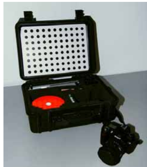
Figure 10: ShapeMetriX3D imaging system consisting of a calibrated SLR camera and changeable zoom lenses.
