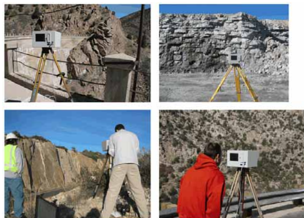
Figure 1. Examples of rock mass characterization using Lidar, a) dam foundation, b) quarry, c) highway, d) mountain environment. Scanner in all images is Optech Ilris 3D
