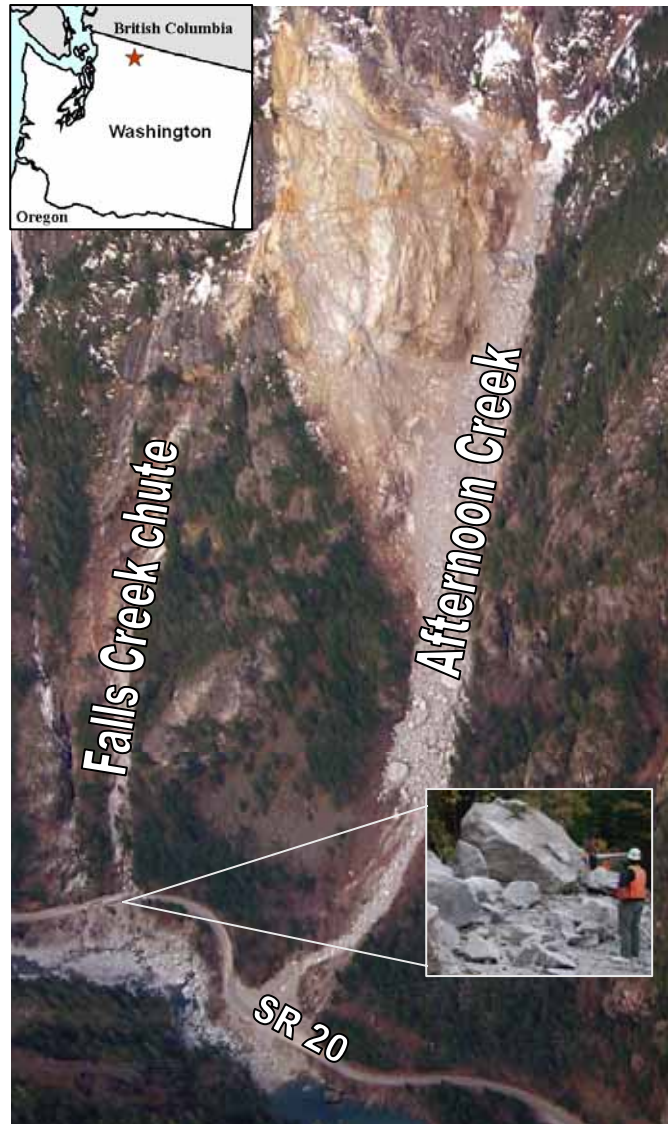
Several traditional methods for characterizing the discontinuity pattern were considered including a scan line and window surveys in the failure zone; however these methods were quickly deemed insufficient as access to important areas near the top of the slope was limited by the steepness of the
