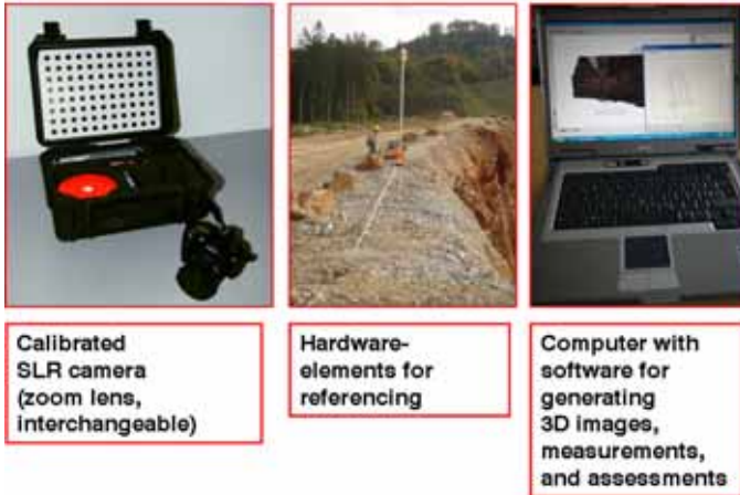
Figure 27: Components of the ShapeMetriX3D system.
