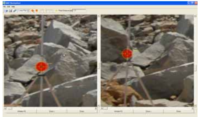
Figure 6: Software component supporting the identification of target points mounted on a range pole.
