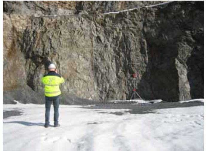
Figure 5 Application of the ShapeMetriX3D system in a magnesite mine. Note that the pictures are taken freehand.
