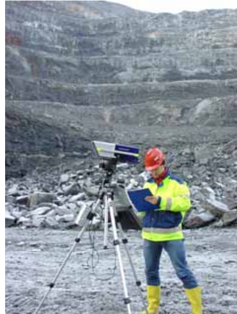
Figure 9: Application of the JointMetriX3D system in an open pit mine in the North of Sweden. Note that a ruggedized portable computer is used in order to control the scanner and save the acquired data instantly.
