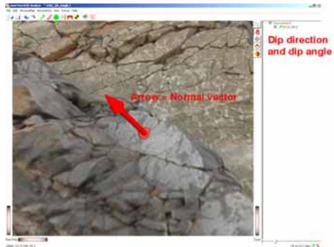
Figure 11: Orientations can be measured at arbitrary locations on the 3D image. Dip angle and dip direction are provided instantly.
