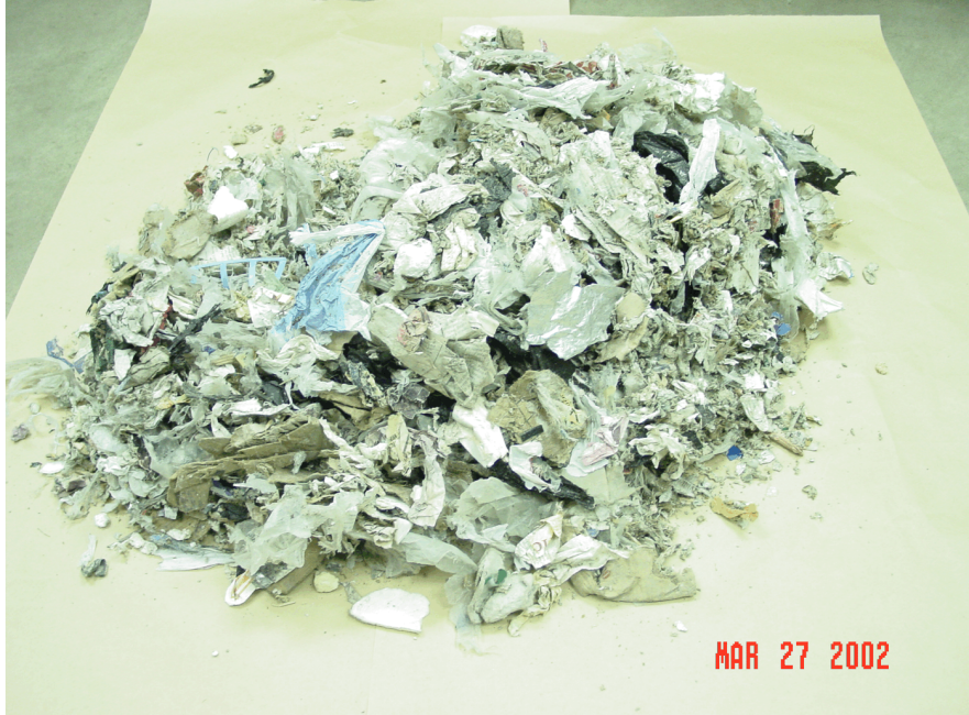
Figure E7. Upgraded -4-inch RDF from air-classifier cleaning.
