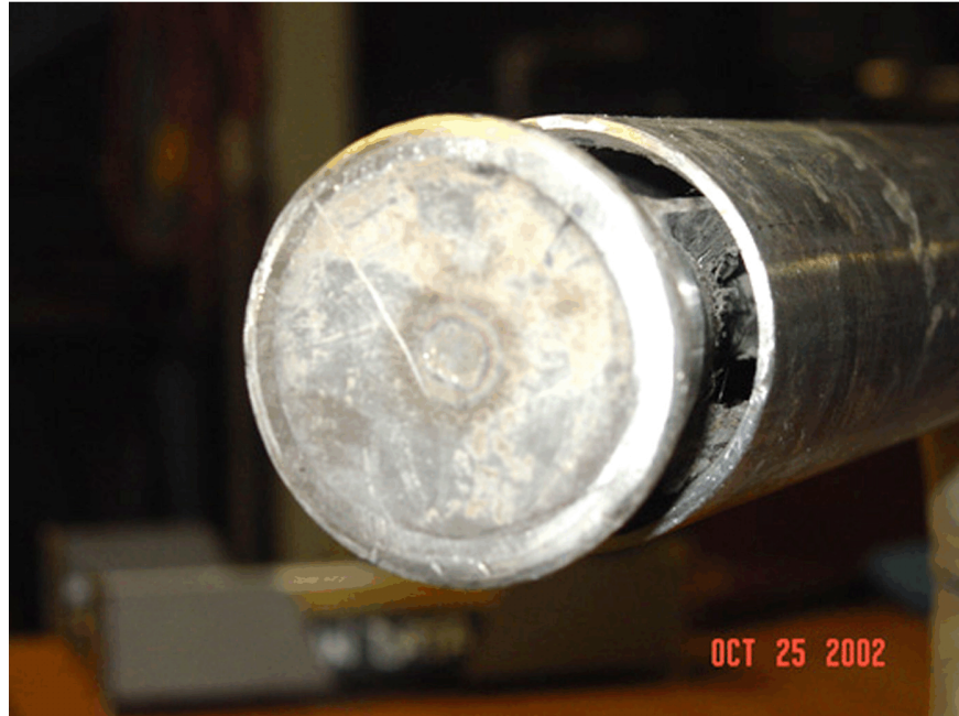
Figure 23. The EERC-2 sludge dispersion nozzle – end view.
