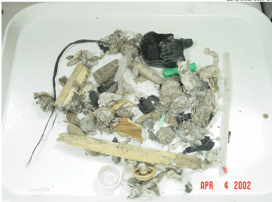
Figure E8. Combustible fraction of heavies from air-classifier cleaning of -4-inch RDF.
