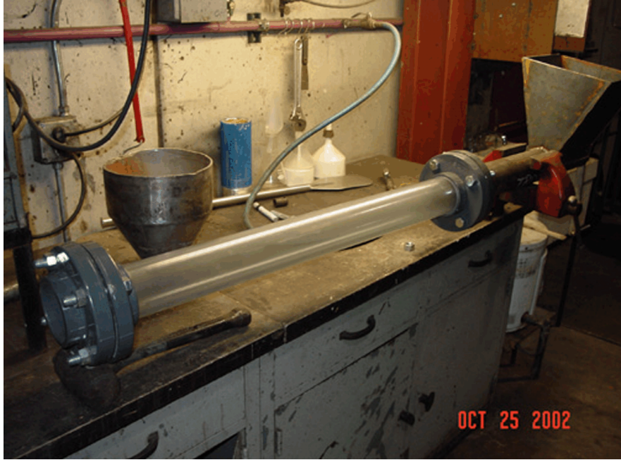
Figure 59. Precompression screw apparatus – transparent material cylinder.
