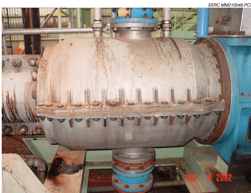
Figure 47. Throat section of plug-screw feeder.
