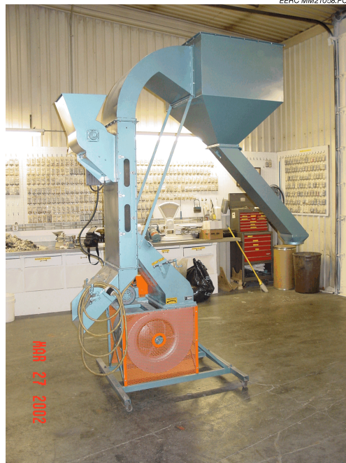
Figure E6. Forsberg air-classifier used for RDF cleaning and biomass entrainment tests.
