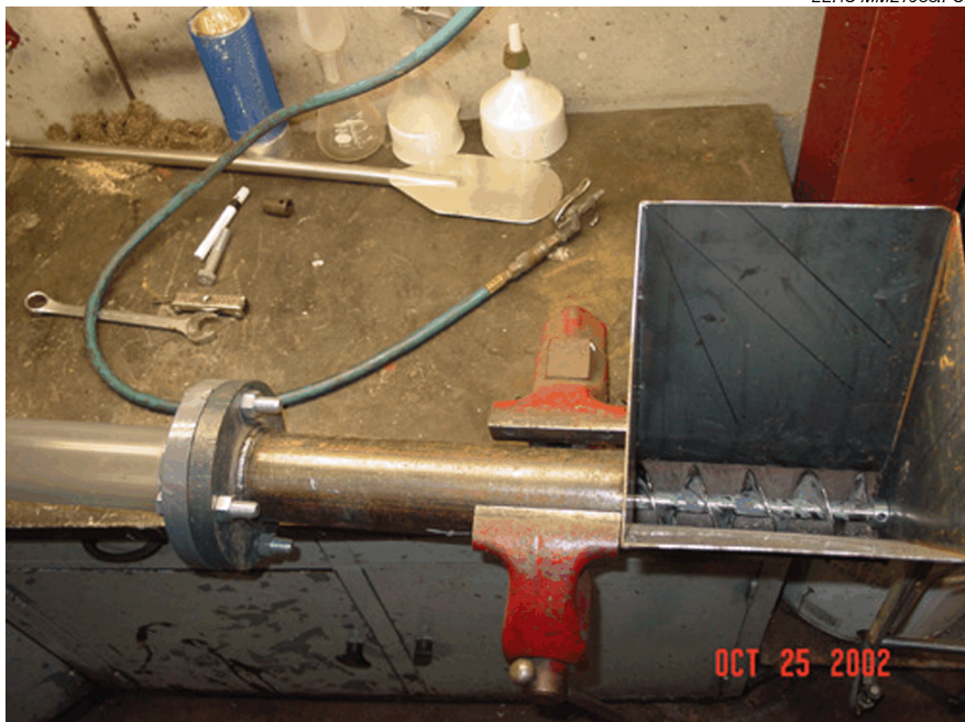
Figure 58. Precompression screw apparatus – feed hopper and compression screw.
