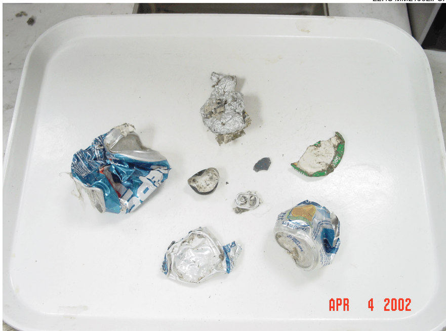
Figure E10. Noncombustible fraction of lights from air-classifier cleaning of -4-inch RDF.
