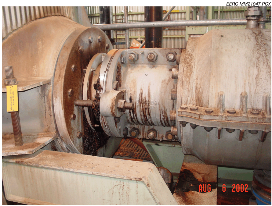
Figure 48. Plug-pipe section in plug-screw feeder.
