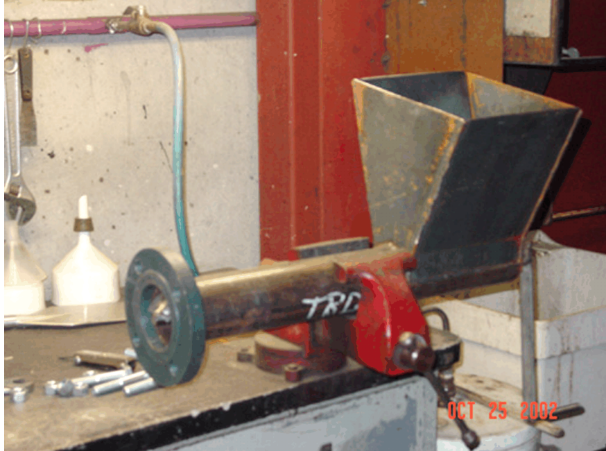
Figure 57. Precompression screw apparatus – discharge of compression screw.
