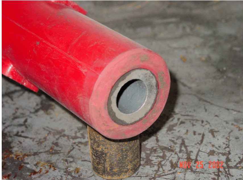
Figure 28. Plug inserted into tip of shotcrete nozzle.
