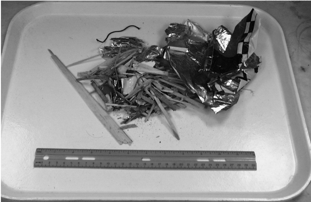
Figure E5. Combined wood, aluminum, ferrous, food waste, glass fraction in NRG RDF.
