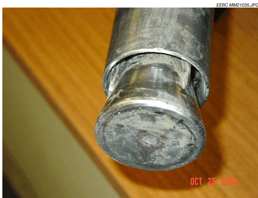
Figure 22. The EERC-2 sludge dispersion nozzle – end view.
