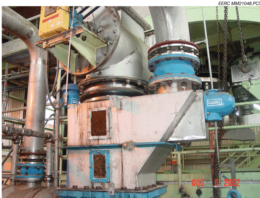
Figure 46. Wood chip-feeding system for plug-screw feeder.
