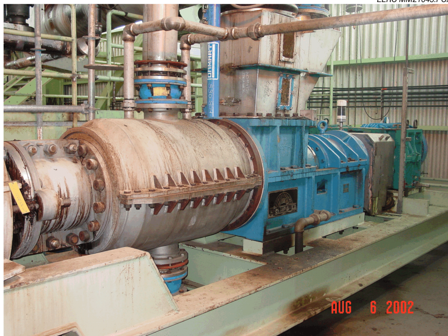
Figure 45. Plug-screw feeder system used in wood chip pulping process.
