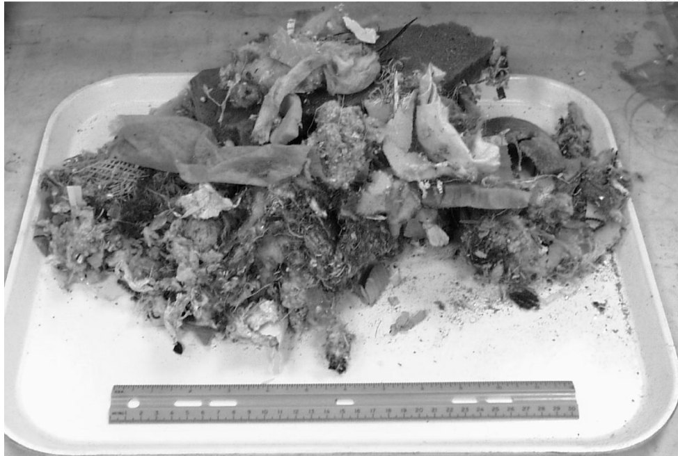
Figure E4. Textiles fraction in NRG RDF.
