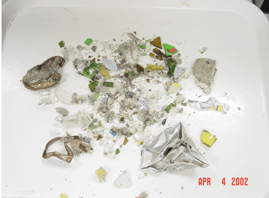
Figure E9. Noncombustible fraction of heavies from air-classifier cleaning of -4-inch RDF.
