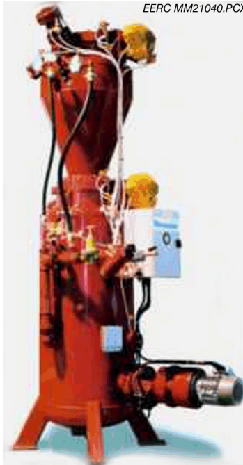
Figure 37. Macawber Controlveyor pneumatic feed system.
