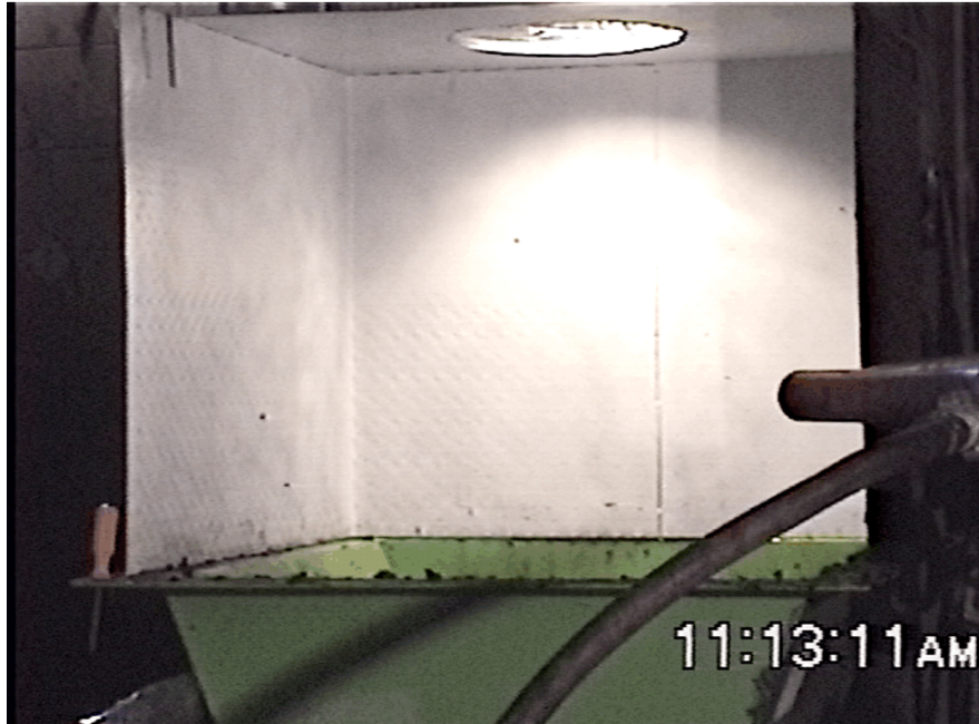
Figure 25. Containment shroud on twin-screw feeder hopper.
