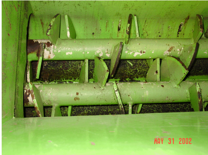
Figure 11. Hopper and overlapping augers of twin-screw feeder.
