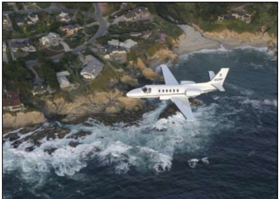
Kip Evans for NOAA Researchers aboard NOAA’s Cessna Citation II twin-jet aircraft used LIDAR to map the coastline of the Monterey Bay National Marine Sanctuary in April.
