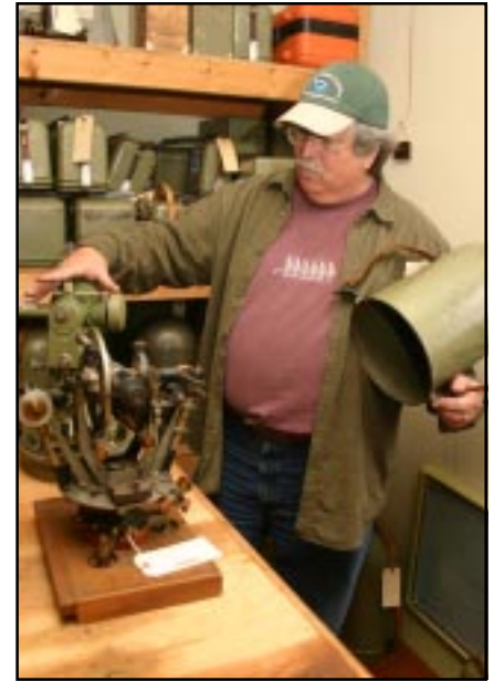
David Hall/NOAA Senior geodesist David R. Doyle uncovers a theodolite that was once used in surveys to measure horizontal and vertical angles.
