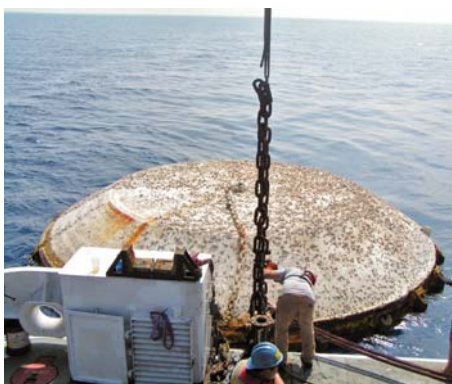
Deck crew attaches a buoy that had flipped over during hurricane Katrina. The buoy was towed to the Data Buoy Center for repairs
