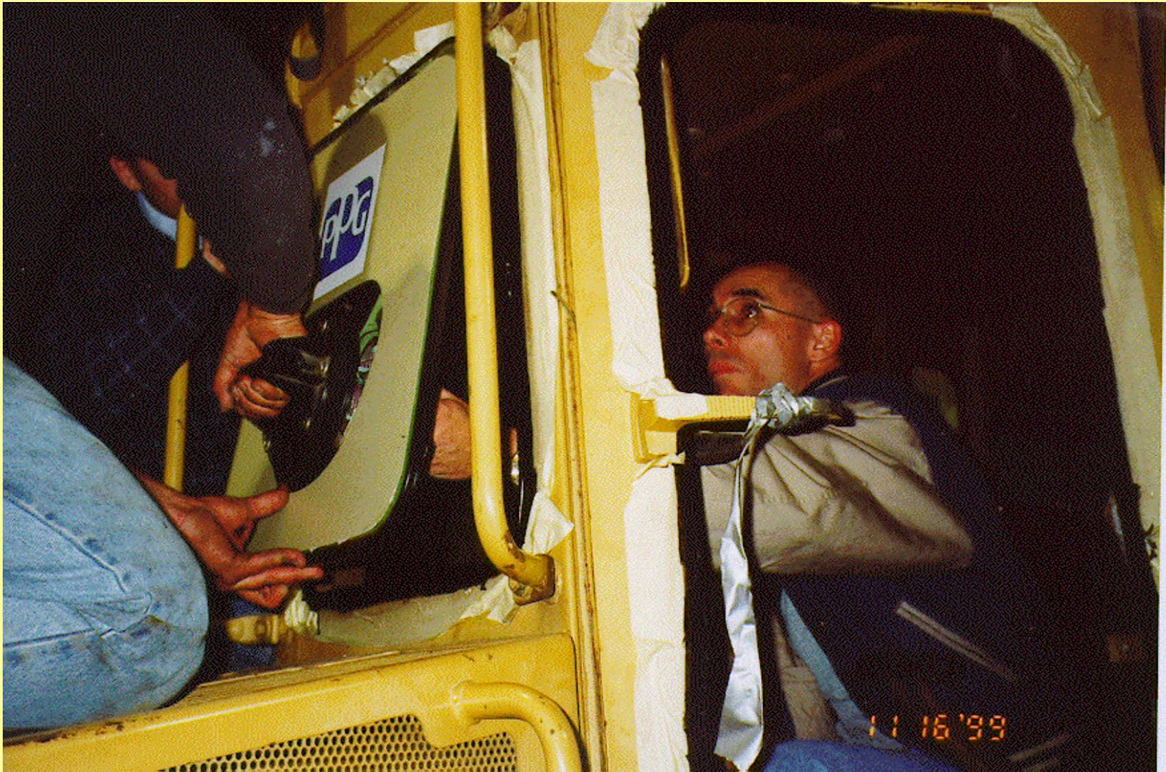
High-strength glass installed using urethane adhesive.
