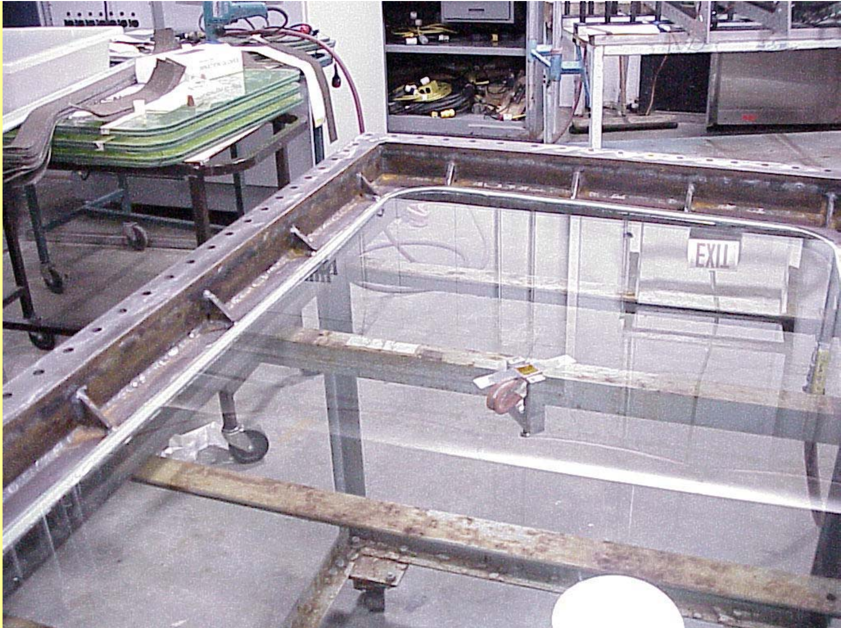
Test fixture - size and shape of D9 rear dozer window
