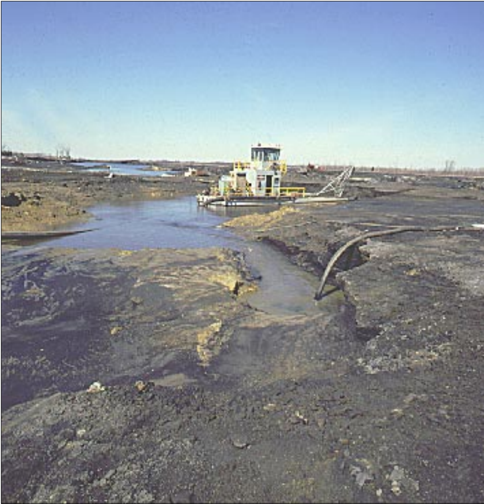
▲ All forms of coal mining are regulated under the Surface Mining Law. This Missouri dredge operation, although very unlike the typical surface mine, must prevent environmental damage during mining and reclaim the site when the operation is complete. The mine operator at this site is recovering coal that was considered refuse at a near-by coal washing facility.
