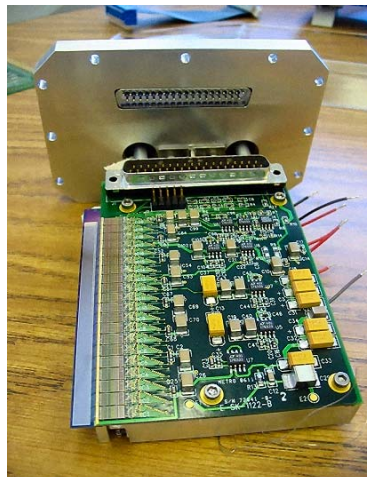
A BNL DETECTOR UNDER DEVELOPMENT FOR DIFFRACTION APPLICATIONS.
