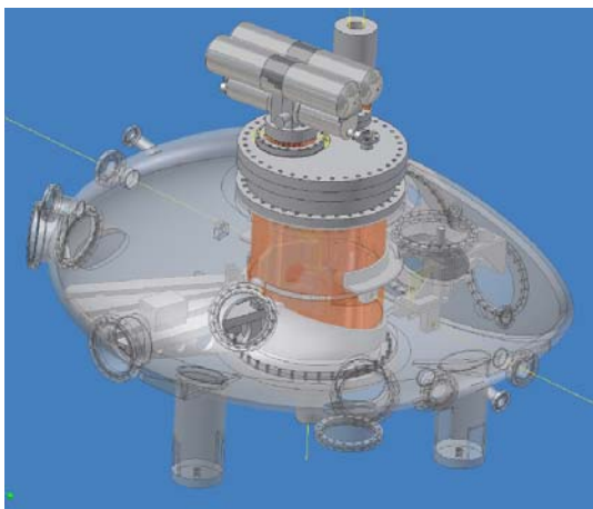
SCHEMATIC OF THE NEW HIGH VACUUM DIFFRACTOMETER AT X13A.
