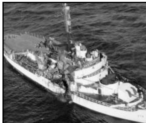
View of damage to the starboard side of the CGC EASTWIND as a result of its collision with the SS GULFSTREAM
