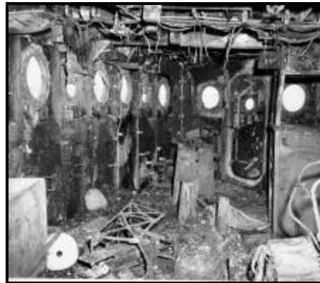
Fire damage to the Pilot House
