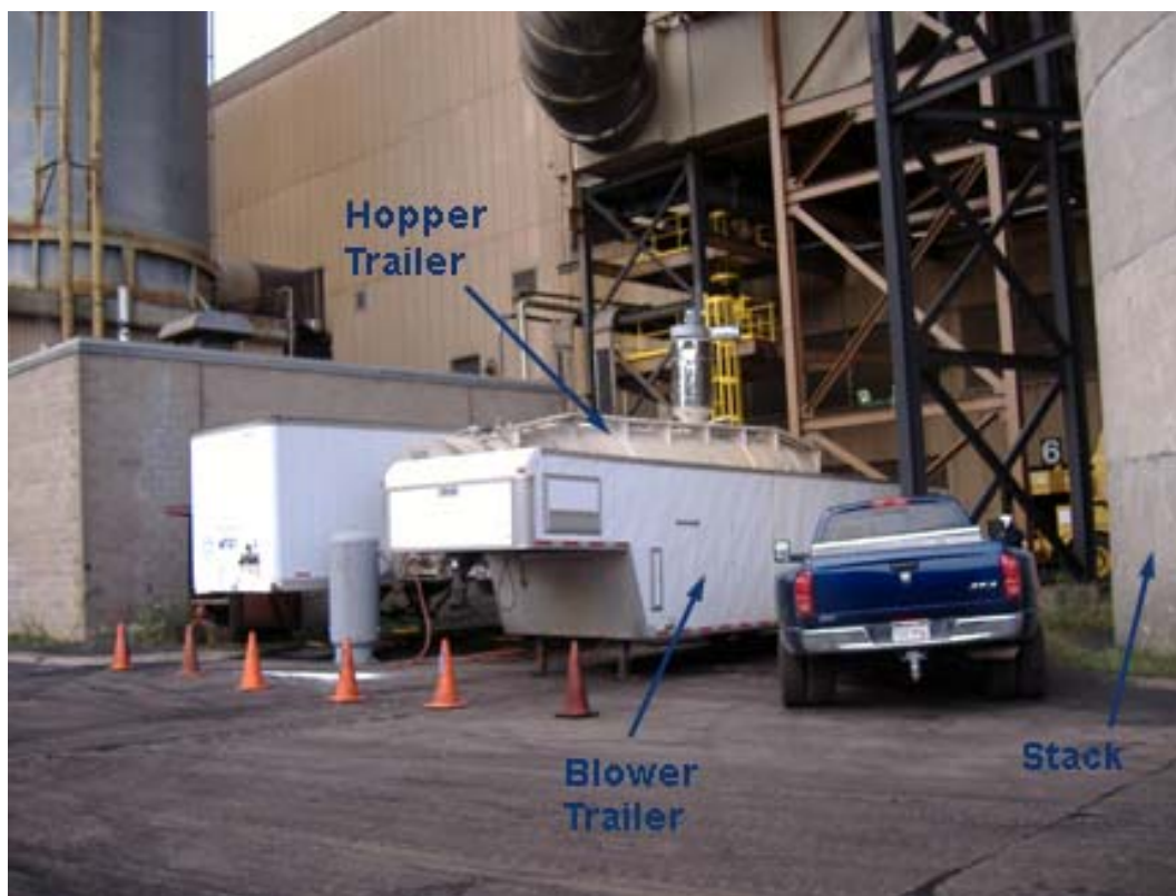
Figure 1. Staging Area for Trona Injection Equipment
