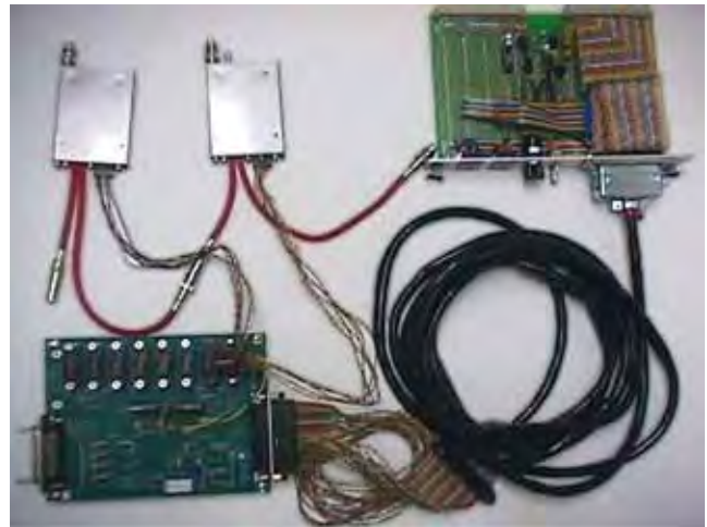
Figure 22: Preamplifier-Amplifier-Discriminator 2 (PAD2) system components.
