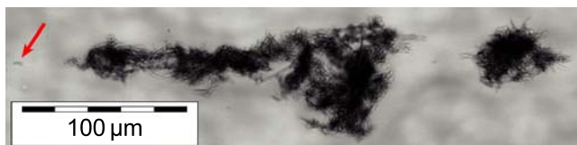
Figure 1: Carbon nanotube clusters suspended in the microfluidic trap in extensional flow in the horizontal direction. The cluster at right has fractured from the main one. Also, an individual tube that has broken from the cluster is visible at the far left (arrow). Individual tubes have also been trapped and examined in flow.
