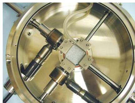
Figure 1: The copper-colored load cells measure the applied force in this biaxial bioreactor. The sample is held in the center of the fixture and can be imaged from below to measure strain. The sample is bathed in nutrients (not shown), and the nutrient is also pumped across the surface of the scaffold through the grips.
