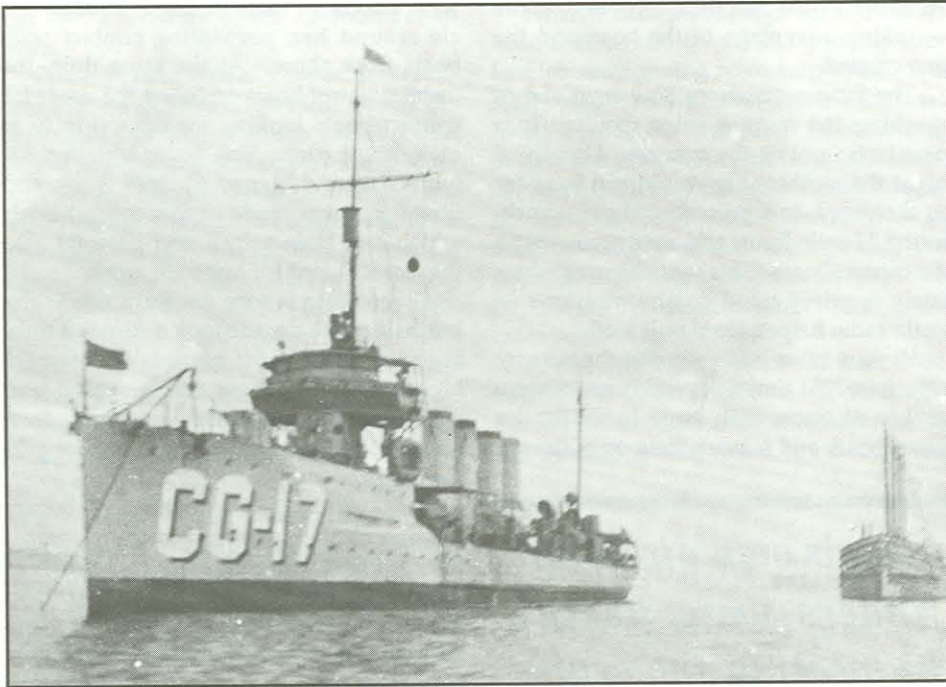
The Coast Guard destroyer Paulding , a 750-ton veteran of World War I, was one of the 25 destroyers temporarily lent from the Navy for Prohibition duties. Fast but uncomfortable and wet in a seaway, Paulding was returned — exhausted — to the Navy in 1931 and “traded” for a flush decker.
