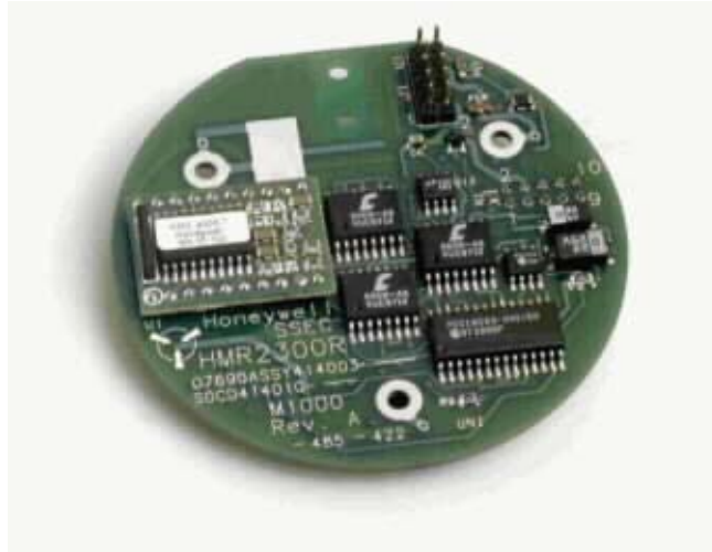
Figure 2.12 Three-axis magnetometer using solid state magnetic sensors (from [14]).
