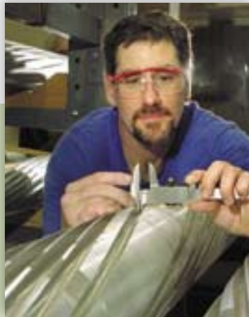
The corkscrew grooves on Siberian Snake magnets help keep proton spins aligned, or polarized.
