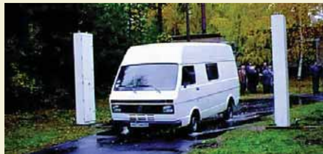
Vehicle portal monitors detect the illegal transport of nuclear and radioactive materials.
