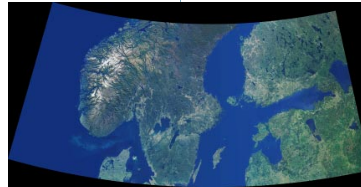
Multi-angle Imaging SpectroRadiometer data were combined with a digital terrain elevation model from the U.S. Geological Survey to create this mosaic of Scandinavia and the Baltic region.
