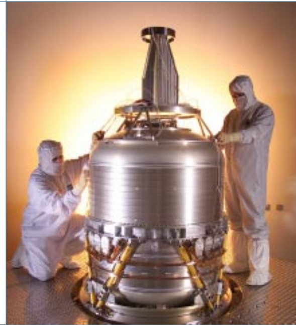
Spitzer's cryogenic telescope assembly is prepared for vibration testing.
