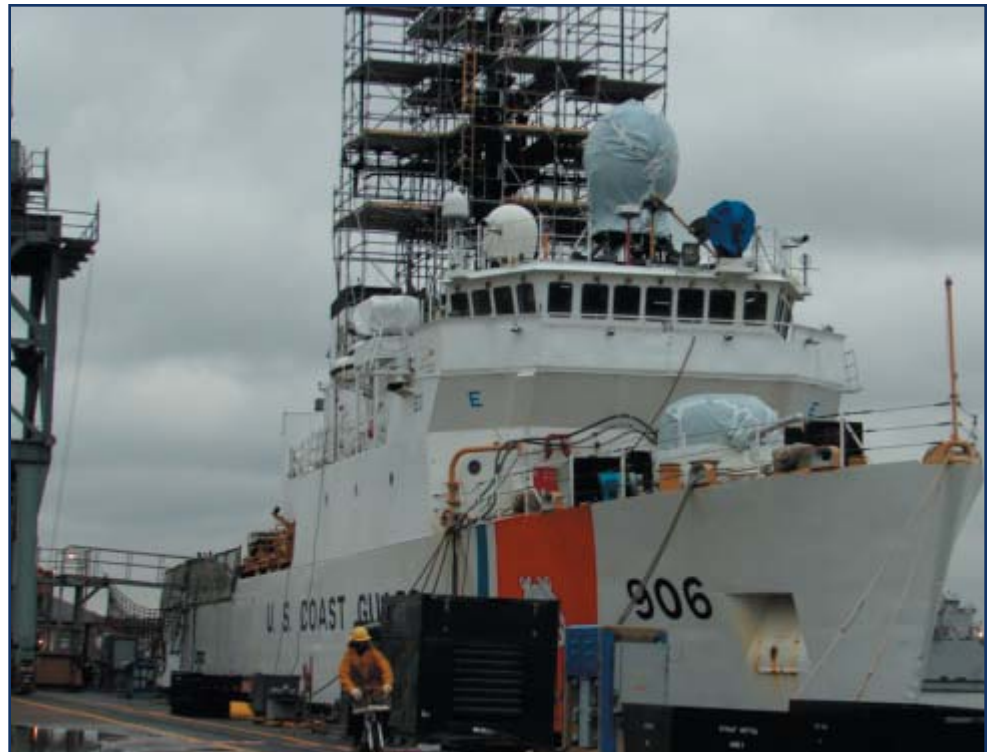
CGC Seneca (WMEC 906) of Boston is a 270' medium endurance cutter now undergoing MEP refurbishment at the Coast Guard Yard, Curtis Bay, Md. (USCG photo)
