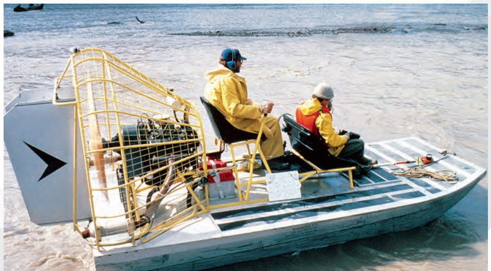
USGS scientists use an airboat to measure the cross section of the Toutle River in Washington State. Accurate, up-to-date measurements are needed to calculate streamflow, develop computer models of surface-water flow, and predict the potential for flooding. Photograph by Pat Pringle, U.S. Geological Survey.
