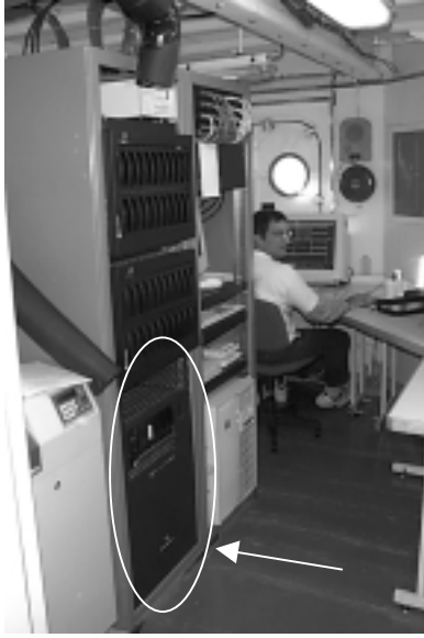
Figure 1 Installation of data management system aboard NOAA Ship RAINIER (SGI Origin 2000 at bottom left of equipment racks)
