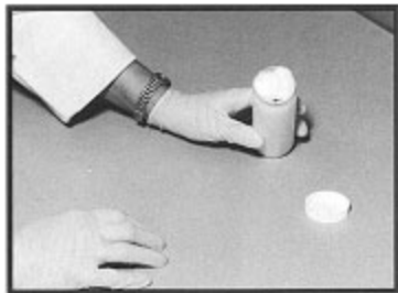
5) Place absorbent on top of tubes and screw on plastic liner cap.
