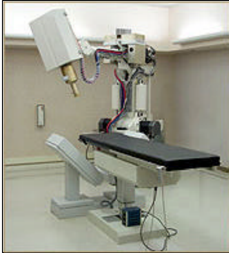
The CyberKnife by Accuray Inc., is an image-guided frameless stereotactic radiosurgery delivery system.
