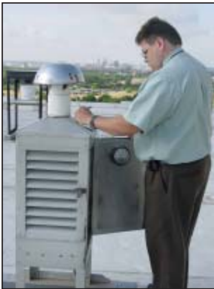
BRC staff member Ruben Cortez uses the ERAMS system to record flow rate and sample times on a weekly basis.
